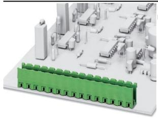
Header, nominal current: 12 A, rated voltage: 250 V, pitch: 5.0 mm, no. of positions: 8, mounting: Soldering
